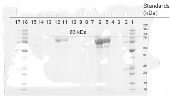
Figure 2: Protein samples from the methanol Fed Batch phase after analysis by SDS-PAGE. Wells were: 1. Standard - dual color; 2. Standard - unstained; 3.4. Enzyme A (52h) - 25µl ; 5. Enzyme A (73h) - 25µl ; 6 Enzyme A (95h) - 25 µl ; 10. Enzyme A (52h) - 5µl ; 11. Enzyme A (73h) - 5µl ; 12. Enzyme A (95) - 5µl ; 16 Standard - dual color; 17. Standard - unstained
