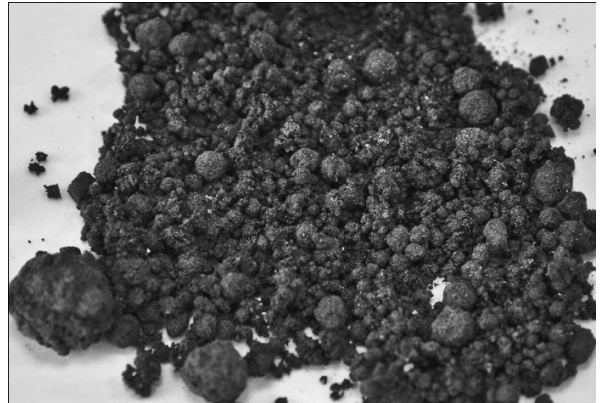
Fig. 7: Clinker nodules, which have been rolling on top of the lining in the crucible.
