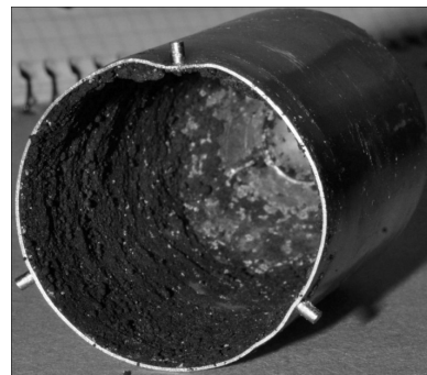
Fig. 8: The inside of the platinum crucible after test burning. Lining of the solid and partly molten material on the walls occurred.
