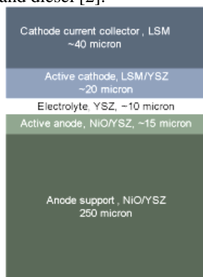
Figure 1: A schematic illustration of an SOFC as produced by Topsøe Fuel Cell A/S [8].
