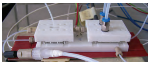
Figure 1.: The continuous membrane microbioreactor prototype
