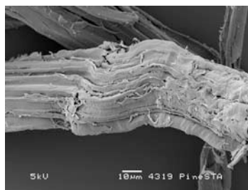
Figure 3: SEM picture of a pine char particle produced in a TGA. The original pine was heated in N 2 at 10K/min to 1373K and was held at this temperature for 30 minutes.
