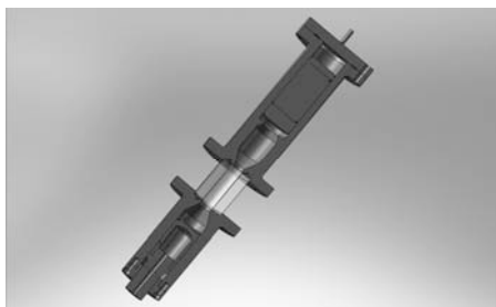
Figure 2: Cut of the new equilibrium cell, where it is possible to see the pistons inside.
