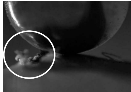
Figure 5: Film sample with a hole, after breakdown (marked with a white circle). Electrode diameter: 2mm.
