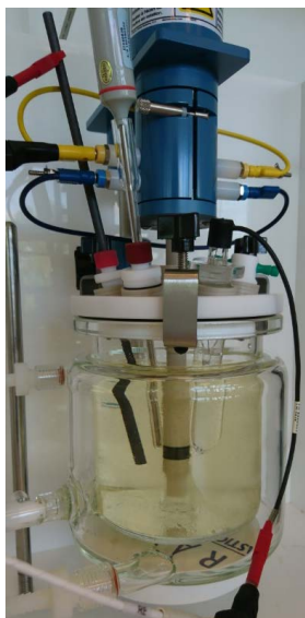
Figure 1: The electrochemical set-up consists of a glass cell containing a solution and a cylinder electrode mounted to a rotating shaft.
