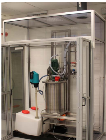
Figure 1: Pilot scale agitated leaching reactor set-up. Coating test panels can be inserted and removed at will inside the reactor
