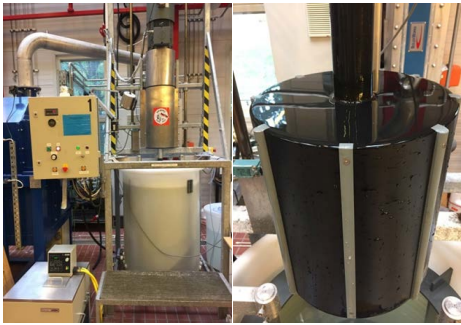
Figure 1: The full pilot-scale rotary setup for drag resistance measurements (left) and the flexible rotor with six artificial welding seams (the grey parts in the photo) on the outer surface (right).
