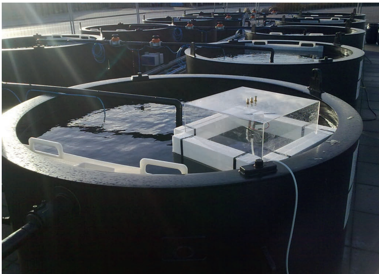
Large cultivation ponds at AlgaeCenter Denmark. The floating incubation chamber is placed in a cultivation pond containing natural seawater and Sea lettuce. Transparent chamber enabled solar light energy to the photosynthesis of the algae. Vigorous air bubbling ensured biomass mixing.
